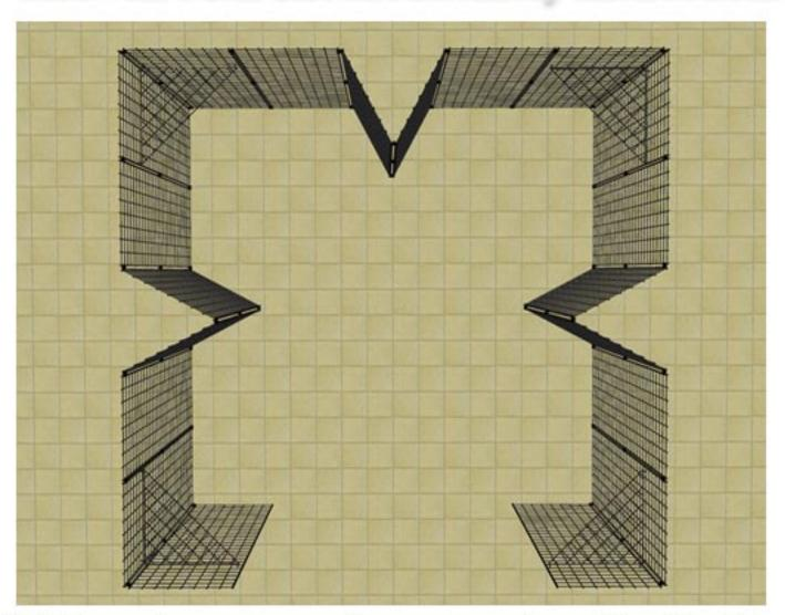
Step 1: With 3 connectors per edge, assemble rear center section consititing of 2 angled panels and 1 panel on each side of angled pair.
