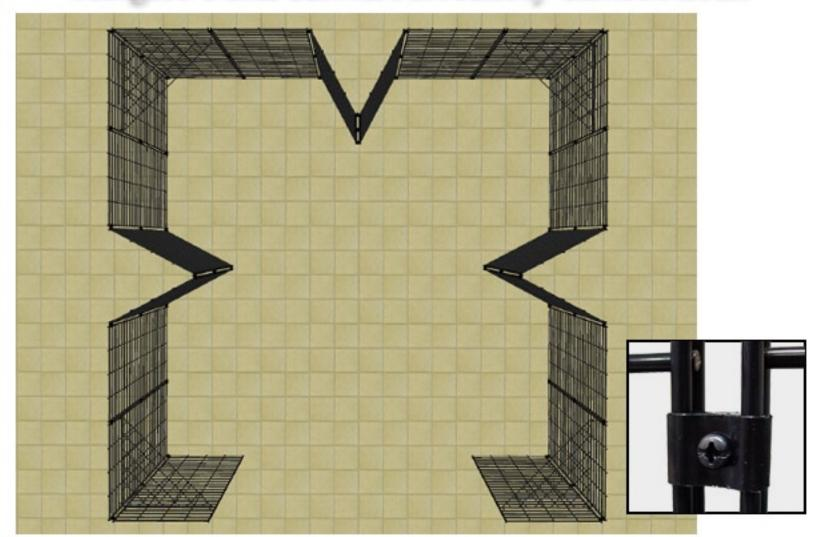
Step 1: With 3 connectors per edge, assemble rear center section consititing of 2 angled panels and 1 panel on each side of angled pair.
