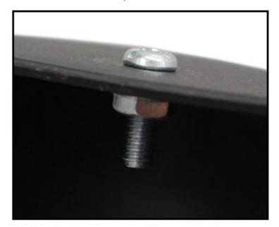
1. Install screw and nut into hang hook hole of form.
