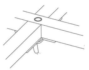
2 SCREW IN WING-NUT AFTER UNFOLDING
