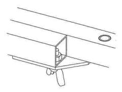
1 UNSCREW WING-NUT & UNFOLD
